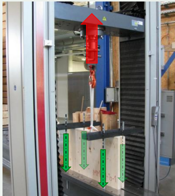
tension test configuration
